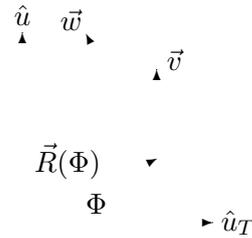
Figure B.1: The *running band* of radius  $R$  is the surface of contact between rock and ice. Here the velocity components, relative to the ice, of a point on the running band are shown.  $v$  is the CM velocity, and  $w$  is the angular component at radius  $R$ . The unit vectors  $(u_T, u)$  coincide with  $(u_x, u_y)$  at time  $t = 0$ . In this case the rock is curling in a counterclockwise sense (so angular velocity unit vector =  $u_z$ ).
