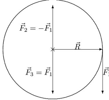
Figure A.1: Force-splitting: The force at the edge  $\vec{F}_1$  can, after adding  $\vec{F}_{2,3}$  be split into a central force  $\vec{F}_3$  and a torque-causing force-pair  $\vec{F}_{1,2}$ . The result is a force  $\vec{F}_2$  in the center of mass and a torque  $\vec{F}_1 \times \vec{R}$ . See [Gre85, P. 142f], [GHS95, P. 34fff].
