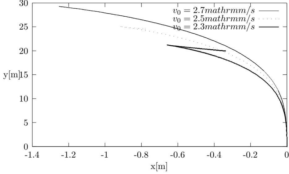
Figure B.2: Approximate curling rock trajectories, calculated from eq. (B.1), eq. (B.2) and eq. (B.4) for three values of initial velocity  $v_0$ . The other parameters are:  $\mu = 0.0127$ ,  $b_{LR} = 0.003$ ,  $\epsilon = 2.63$ ,  $R = 0.065$ .
