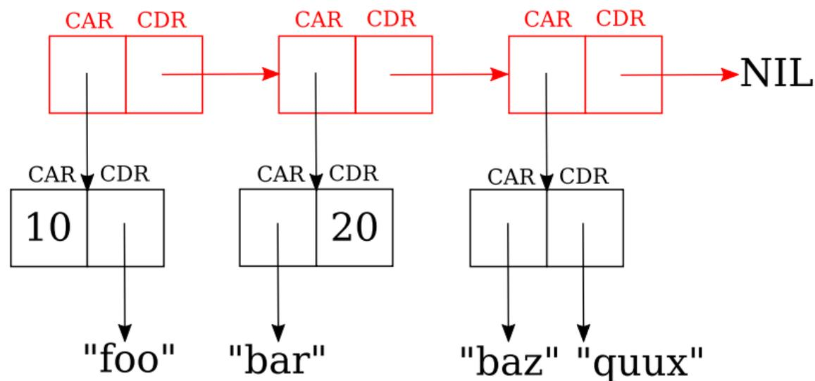
This is the in-memory representation of the dictionary  $\{(10, \text{"foo"}), (\text{"bar"}, 20), (\text{"baz"}, \text{"quux"})\}$ . The entries form a list of complex data (the *spine* of the dictionary).
