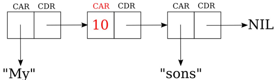
This is the in-memory representation of the list ["My", 10, "sons"] using CONS cells. Primitive data is stored in the CAR of the relevant cell as before.
