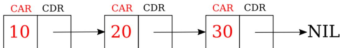
This is the in-memory representation of the list [10, 20, 30] using CONS cells. Each CONS cell is one list node. CARs contain the data.
