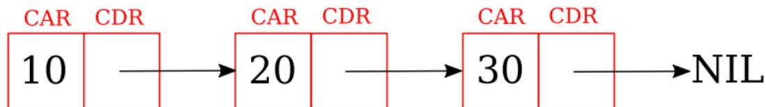
This is the in-memory representation of the list [10, 20, 30] using CONS cells. Each CONS cell is one list node.
