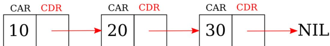
This is the in-memory representation of the list [10, 20, 30] using CONS cells. Each CONS cell is one list node. CARs contain the data. CDRs contain references to the next list node, or NIL for the end.
