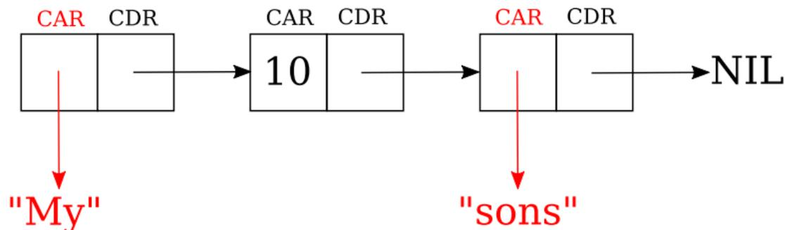
This is the in-memory representation of the list ["My", 10, "sons"] using CONS cells. Primitive data is stored in the CAR of the relevant cell as before. Complex data is stored elsewhere, and the CDRs of the relevant cells store references to that data instead.
