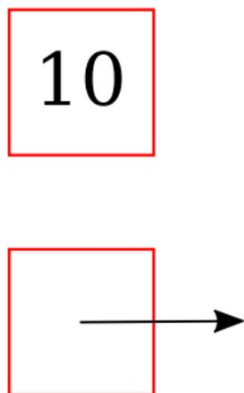
We represent machine words using boxes. Adjacent boxes are adjacent machine words in memory (these two are not).
